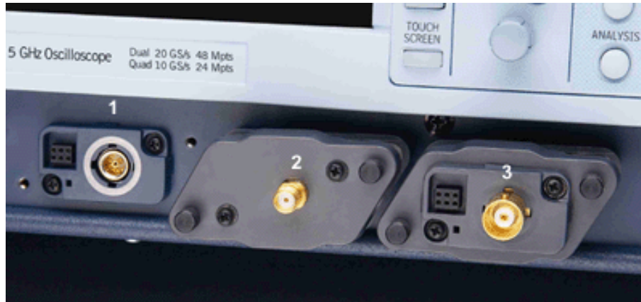
(1) BMA Female Connector; (2) ProLink BMA-to-SMA Adapter Installed; (3) ProLink BMA-to-BNC Adapter Installed
