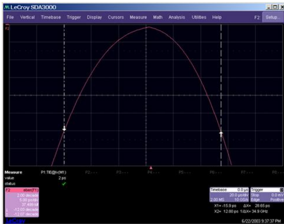
Figure 9. Total jitter curve. The vertical values of this curve represent the probability of a data transition occurring at a time represented by the horizontal axis. The horizontal center of the plot is 0 ps. The two markers are placed at the vertical level corresponding to a bit error rate of 10 \times 10^{-12} and the horizontal distance between these two points is the total jitter at this bit error rate.
